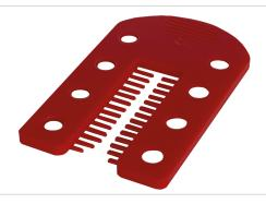
Knudsen Fix Shims spacer blocks are suitable for all types of tasks where items need to be stabilized, e.g. when installing doors and windows, setting up kitchen and bathroom elements, moldings, panels, etc. As the Fix Shim is designed as a split piece with fins, which ensures a stable grip on the screw during any assembly, it is particularly suitable for mounting on vertical surfaces. Fix Shims cannot be used for heavy leveling tasks such as floors, rafters etc.
